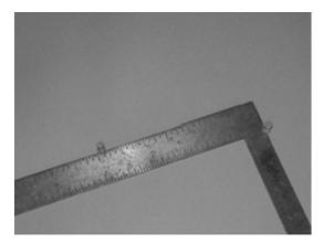
This is a very interesting tool used by carpenters. Carpenter's squares have metric and imperial measurement scales along both sides. The square has many applications. One of them is to copy angles by using the markings along the scales. Note that in your own geometry set, you probably have two set squares, as described earlier, and which can be used like a carpenter's square, as shown in the following example.
