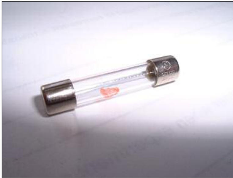
good fuse (clear wire is connected from each silver cap)
