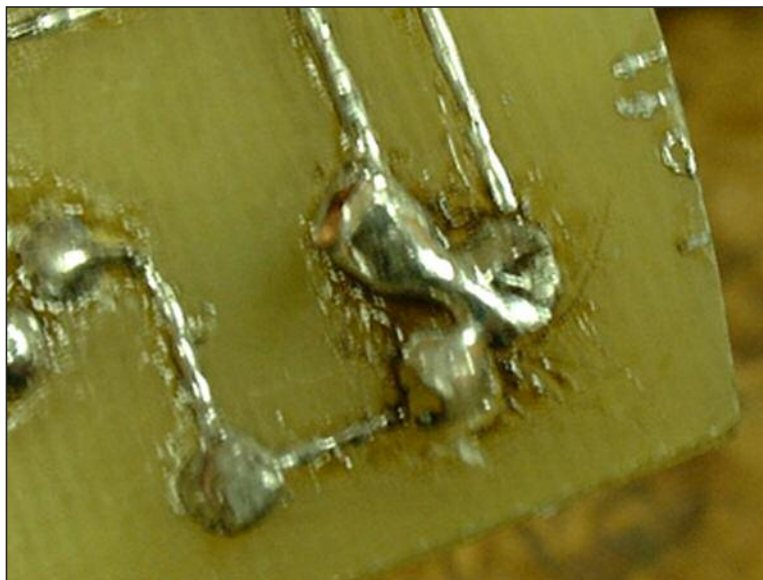
picture of a poor solder joint (too much solder)
