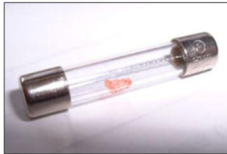
fuse (close up)
