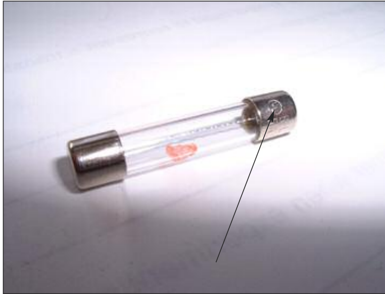
fuse amperage and voltage rating stamped here
